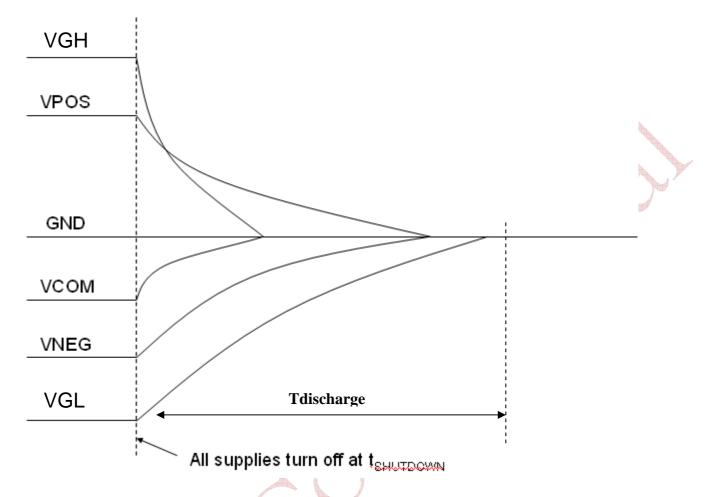
Note8-1 : Supply voltages decay through pulldown resistors.
