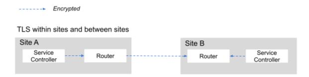
The Understanding TLS traffic between applications and routers section describes TLS traffic between a client and the router in a site, and then between the router and the server in a different site.
