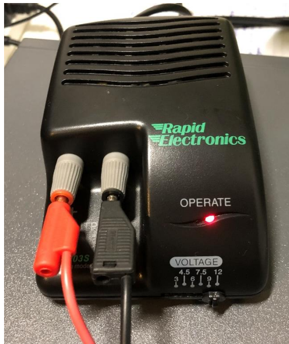
Figure 88 - Rapid Electronics 12V DC power supply that was used for this circuit
