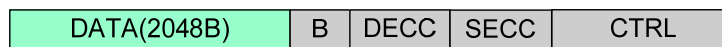
Figure 4-37 Data storage structure of the NAND flash with the page size of 2 KB (2048 + 64 bytes) in 1-bit ECC mode
