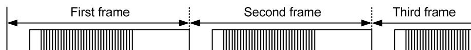
Figure 13-25 Frame format for transmitting NEC with full repeat codes by pressing the key continuously
