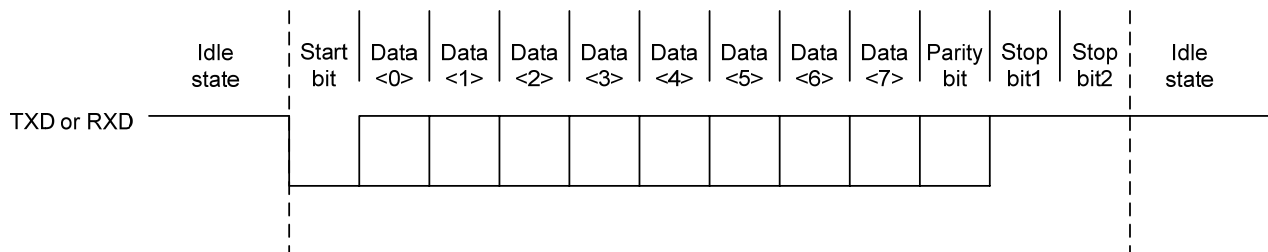
Figure 13-18 Frame format of the UART
