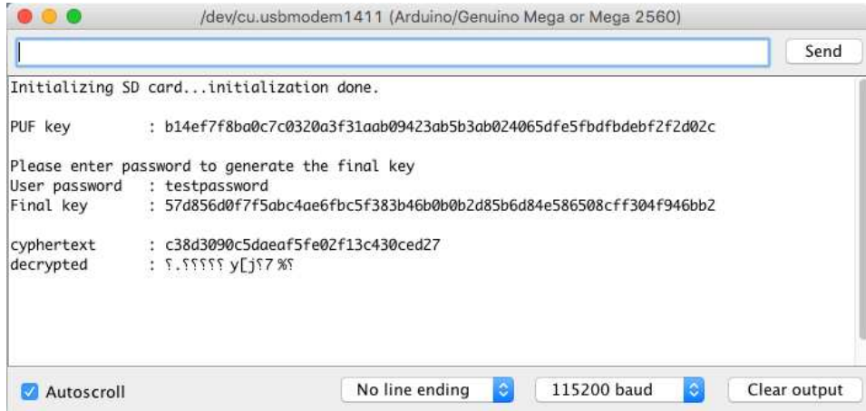
Figure A.8: Screenshot of the bitcoin key storing experiment during decryption stage. The bitcoin key 'testpasswordtest' is previously secured by using SRAM Cypress CY62256NLL 'B' and user's password 'testpassword'. The bitcoin key cannot be reconstructed because the SRAM utilized for the decryption is SRAM Cypress CY62256NLL 'A'.
