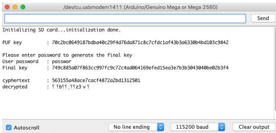
Figure A.11: Screenshot of the bitcoin key storing experiment during decryption stage. The bitcoin key 'testpasswordtest' is previously secured by using SRAM Cypress CY62256NLL 'C' and user's password 'password'. The bitcoin key cannot be reconstructed because user's password is wrong.
