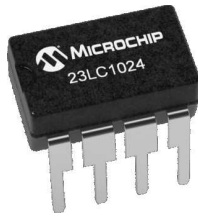
Figure 4.1: SRAM Microchip 23LC1024.
