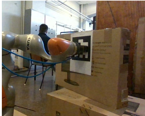
Figure 4.5: Approximate validation of position by aligning the gripper center to the center of the ArUco marker, then marker center position is measured. Results are in Table(4.1).
