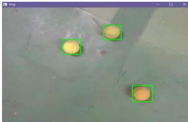
Fig. 6 Detection of balls using Haar Cascading
