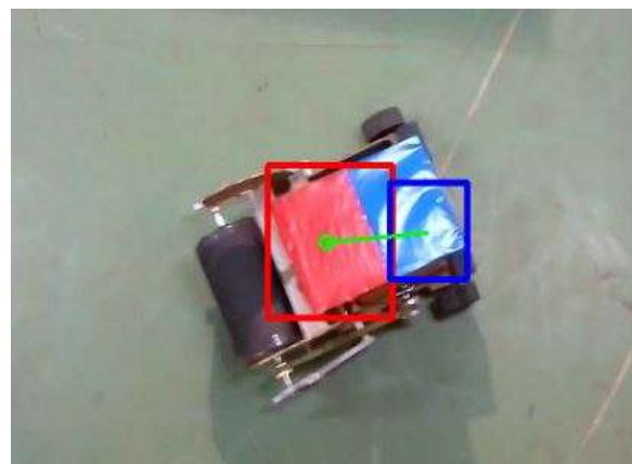
Fig. 13 Roller mechanism engulfs the ball inside the robot.
