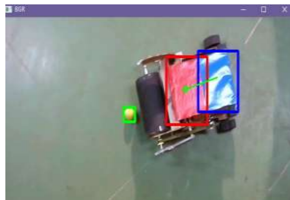
Fig. 12 Traversal of robot towards the ball.
